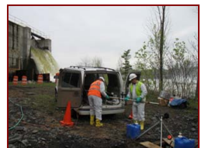
Late in the day on the river – borehole geophysical logging by a spillway
